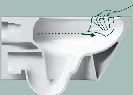
The newflush® water vortex optimises flushing performance and significantly reduces the sound of toilet flush.
