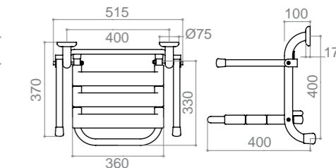
**RIBALTABLE PER DOCCIA CON SCHIENALE SEDUTA IN PE, STRUTTURA INOX**
